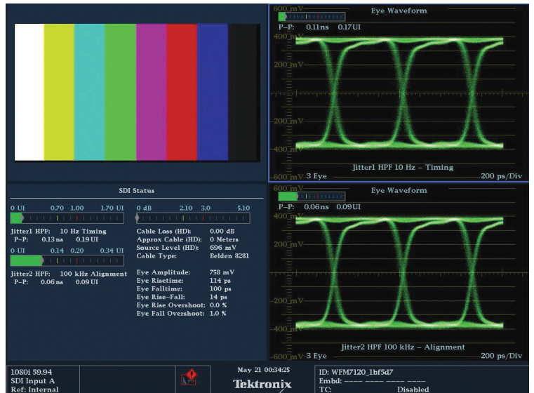
[Timing Jitter와 Alignment Jitter 측정]
