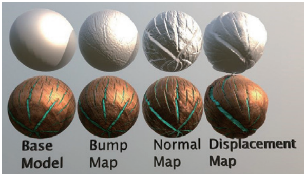
Differences between Bump vs Normal vs Displacement BY SPIDERLILI
