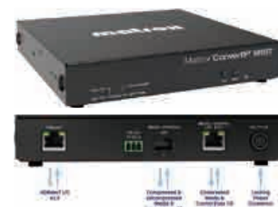
ConvertIP SRST Single-channel RJ45 HDBaseT™-to-IP transmitter/receiver
